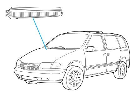
The odor and particulate air filtration system is designed to reduce the concentration of objectionable exterior odors as well as airborne particles such as dust, spores and pollen in the air being supplied to the interior of the vehicle. The extent of EXTERIOR odor reduction depends on the odor itself and the perceptional threshold of the individual. The odor and particulate filtration system gives the following benefits to customers:
